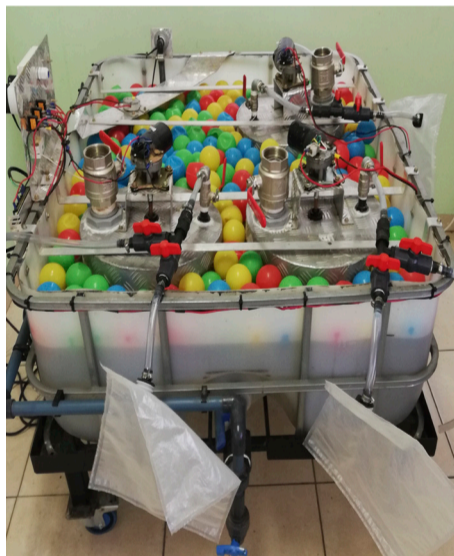
Pilot anaerobic bio-digester plant housed at NUST's IDL.
